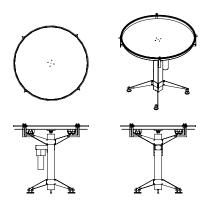
The MDT, medium duty turntables are used wherever product accumulation off of a conveyor line is required. Stationary guide rail is Product is For example-
