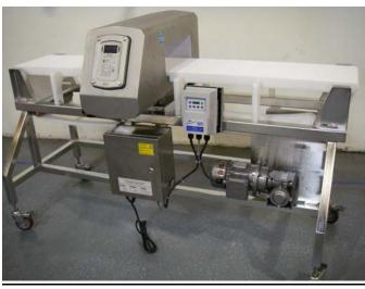
The MDC (Metal Detector Conveyor) offers a washdown solution for maintaining a metal-free product in a GMP abiding plant.
