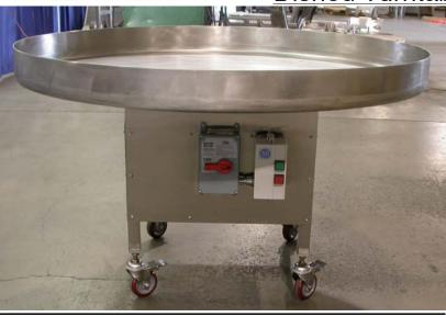
The dished turntables are used wherever product accumulation after it exits wrapping and bagging machinery is required. For example-
